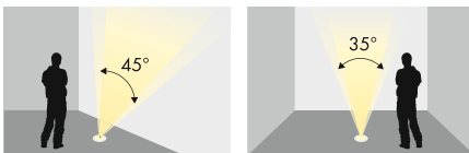
Asymmetrische Linse 45°/35° / Asymmetrical lens 45°/35°
